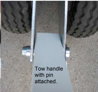
Tow handle attached to tank
