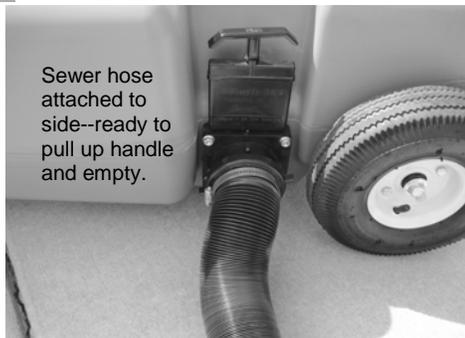
Sewer hose attached to side--ready to pull up handle and empty.
