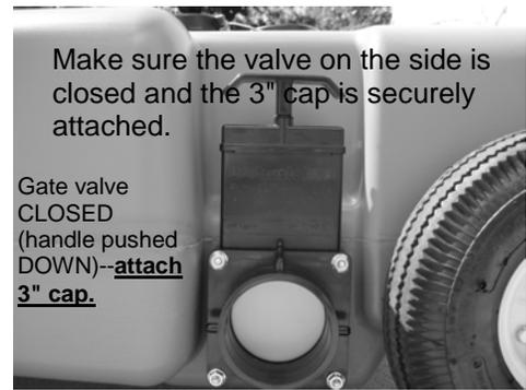
Make sure the valve on the side is closed and the 3" cap is securely attached.
