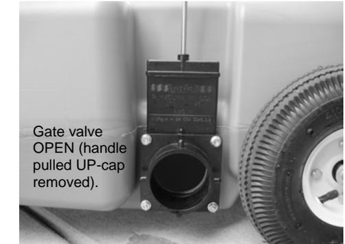
Gate valve OPEN (handle pulled UP-cap removed).
