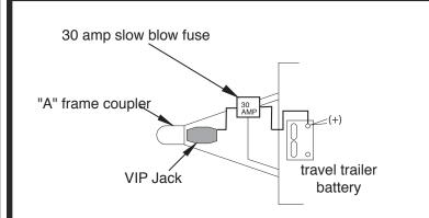
Connect the lead-wire directly to the positive (+) lead of the travel trailer's battery using a twelve (12) gage wire. Be sure the connection is a good one.
